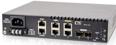
The next generation Carrier Ethernet Network Interface Device (NID) is designed for business connection in Ethernet virtual connection technology. The MSW-4204 is equipped with 2 SFP+ slots, dual rate 1G/10Gbps and 4 ports Gigabit RJ45 network interfaces. It can be configurable as either UNI or NNI device which are CE(Carrier Ethernet) 2.0 compliant for Metro Ethernet network deployments.
